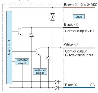
\*The D2 F-TS D slave unit does not have power supply wires (brown/blue) because power is supplied from the master unit.
